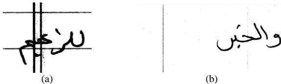
Fig. 2. (a) Ruled vertical lines affecting text. (b) Noise-generated lines.
