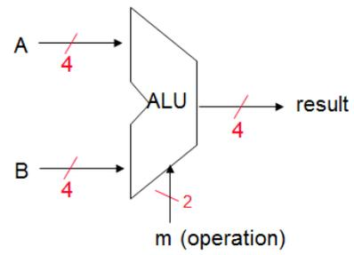
a) Design a one-bit ALU slice that performs these three operations. Use full adder, multiplexer, and basic logic gates as your building blocks.
