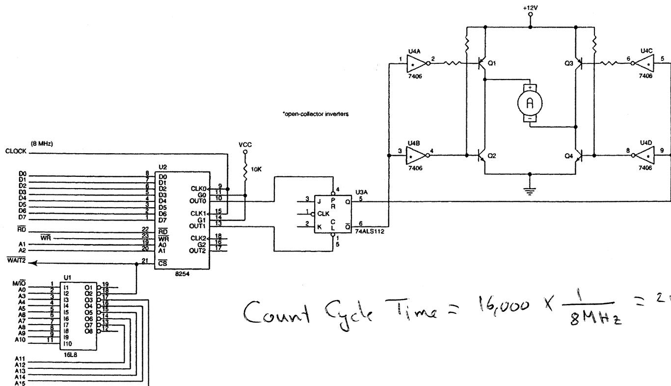
$$\text{Count Cycle Time} = 16,000 \times \frac{1}{8\text{MHz}} = 2\text{ msec}$$
