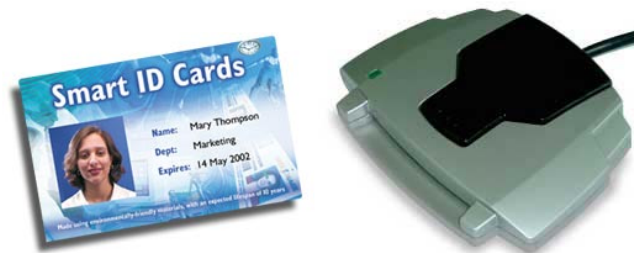
Figure 12: Smartcard (ACOS3-32) and smartcard reader (ACR38)
