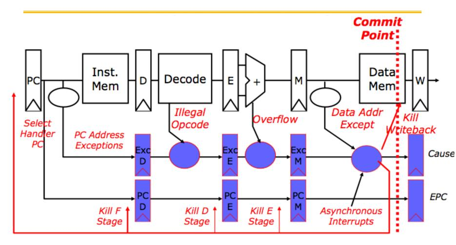
Key observation: architected state only change in memory and register write stages.
